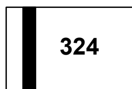
324= Device Marking Code Bar denotes Cathode
